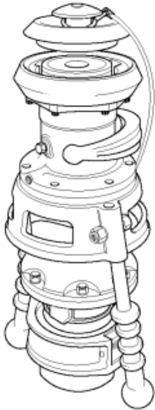
Example of a pressure refuelling nozzle.
